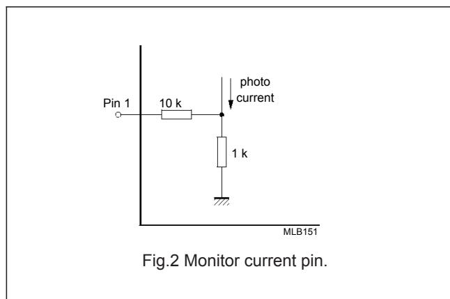
Fig.2 Monitor current pin.
